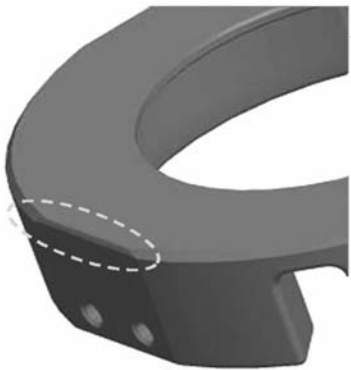
(b) 线圈基底的修改设计 (b) Modified design of coil base
